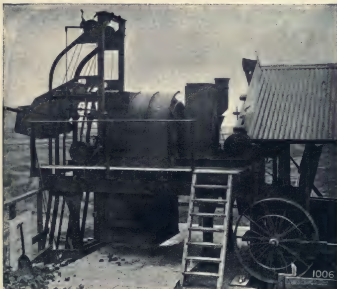
A RANSOME DRYER SUPPLIED TO THE WEST HAM CORPORATION FOR GRAVEL DRYING.
